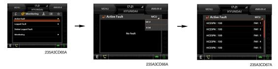
· The active faults of the MCU, ECM, AAVM (option) can be checked by this menu.
