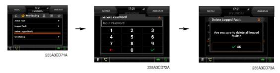
· The logged faults of the MCU, ECM, AAVM (option) can be deleted by this menu.
