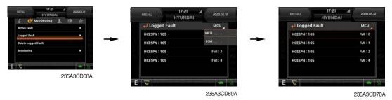
· The logged faults of the MCU, engine ECM can be checked by this menu.
