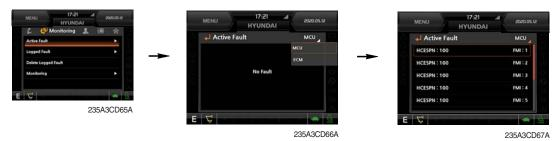
· The active faults of the MCU, engine ECM can be checked by this menu.
