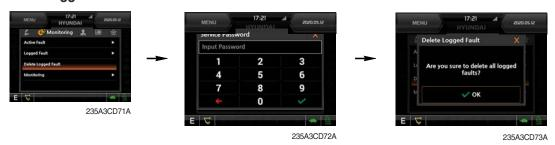
· The logged faults of the MCU, engine ECM can be deleted by this menu.
