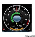
① This displays the engine speed.
