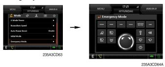
· This mode can be used when the switches are abnormal on the cluster.
