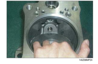
(4) To pump casing (271, 272), fit drive shaft (111, 113) set with bearing (123), bearing spacer (127) and stop ring (824).
